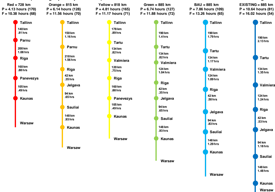
Figure 3 – Distance/passenger journey time comparison with the Business As Usual case scenario and the Existing Service.
