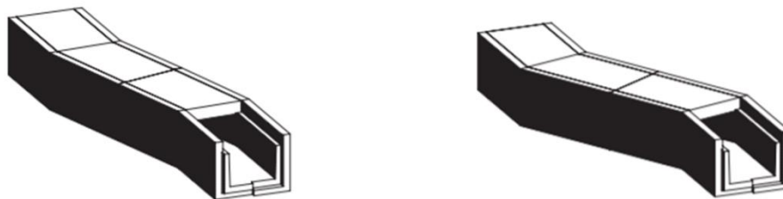
Cable channel elements; 15 degree turn (left) and 30 degree turn (right).
