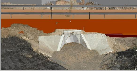
BIM and Lidar integration allows a quick and simple comparison between what has been designed (BIM) and what has been built (Lidar)
