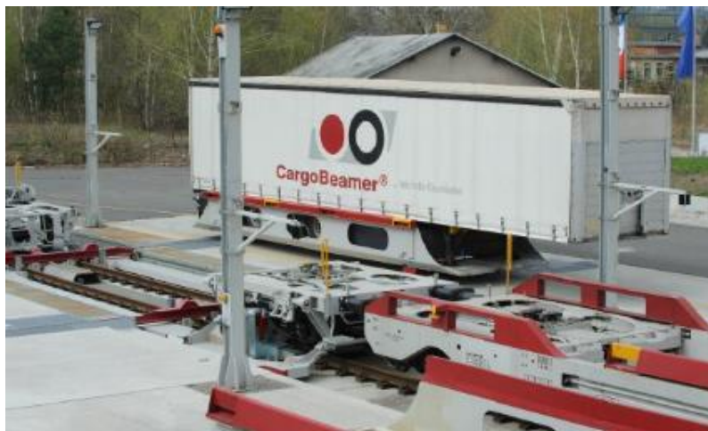
Illustration 33. Horizontal loading using CargoBeamer solution
