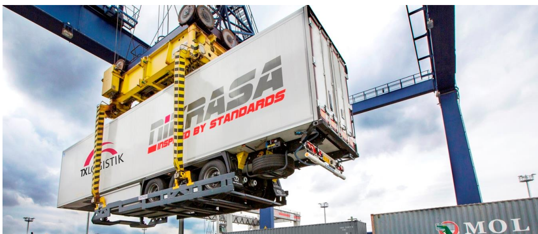
Illustration 2. Lifting non-craneable semi-trailer using a supporting platform (source NiKRASA system)
