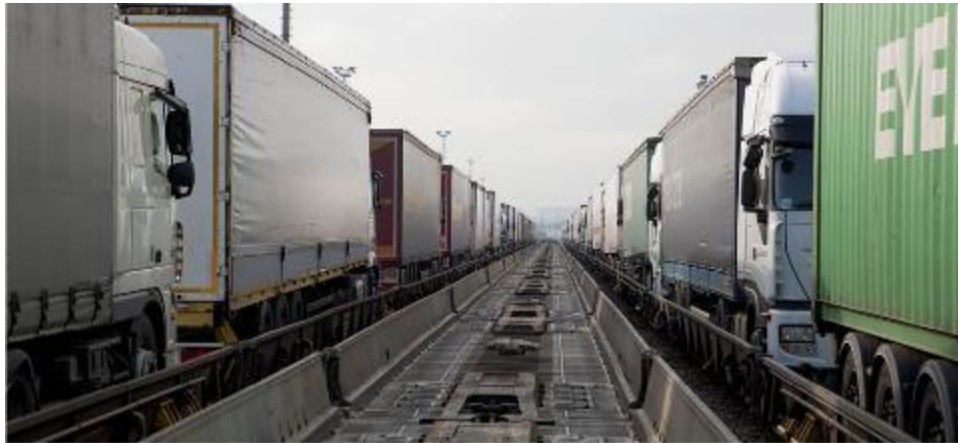
Illustration 6. Low floor flat wagon (source RALpin).
