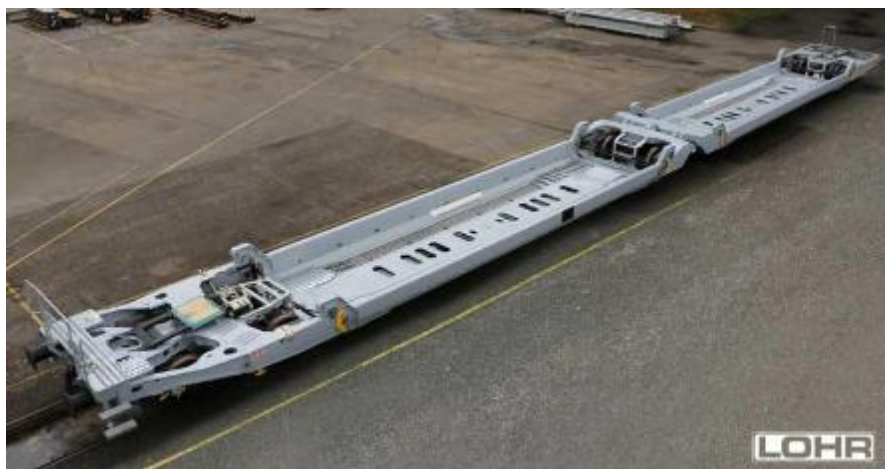
Illustration 30. Modalohr wagon with extra low floor.
