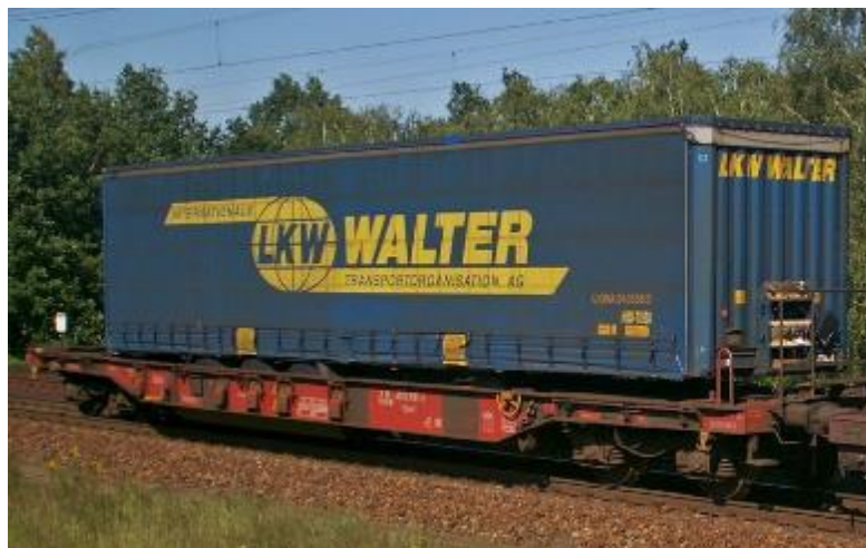
Illustration 9. Conventional pocket wagon for semi-trailer
