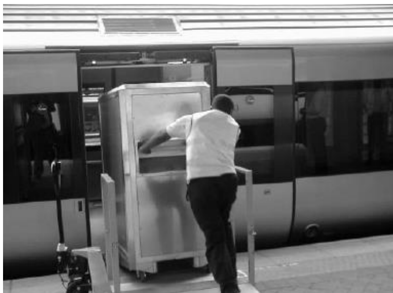
Illustration 25. Carrying and loading luggage on train board using a rolling container + Pallet truck handling device
