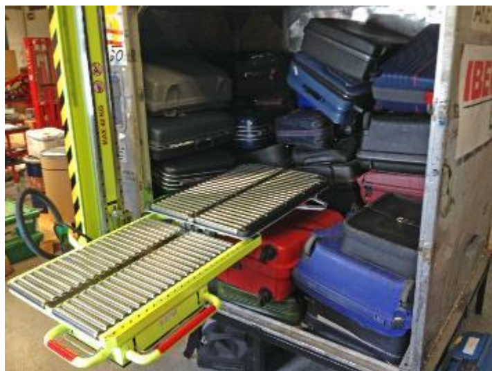
Illustration 28. Container equipped with a telescopic table
