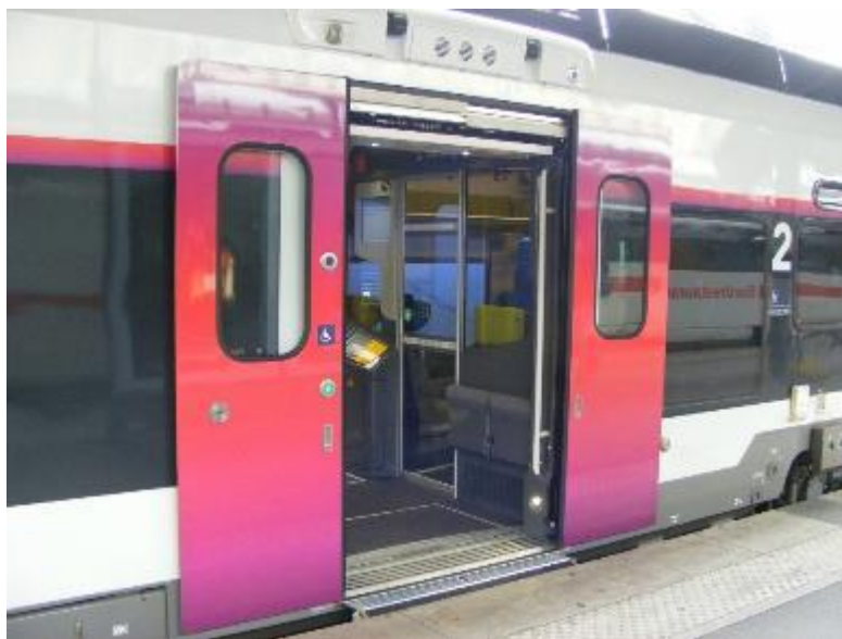
Illustration 29. Direct access to 760 mm height platform (Coradia)
