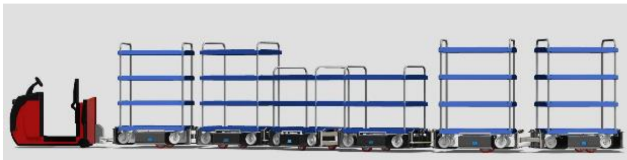
Illustration 26. Tug for the transport of containers or trolley cages with lifting system integrated in the wagon
