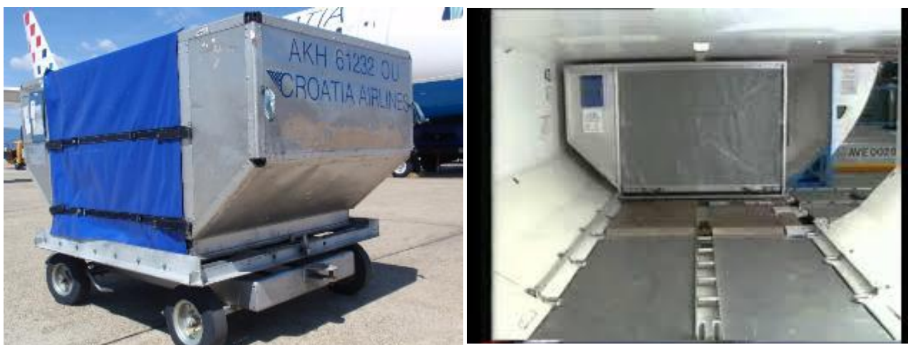
Illustration 22. Aircraft container, loaded into plane and locked
